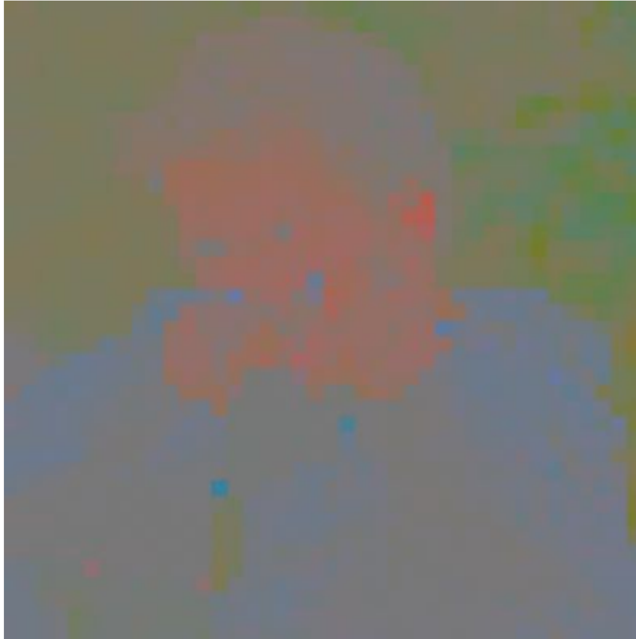
Contents of CbCr color channels downsampled by a factor of 20 in each dimension (400x reduction in number of samples)
