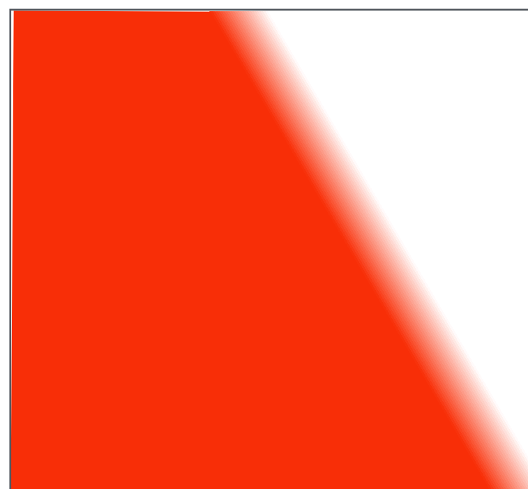
Reconstructed signal (lacks high frequencies)
