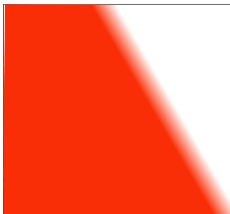
Reconstructed signal (lacks high frequencies)
